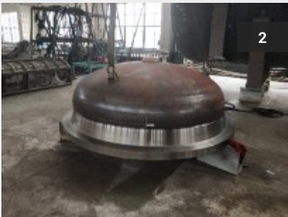
Picture 1 – Forming of Shaft Cap
