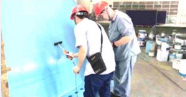
100% LOW VOLTAGE CONTINUITY TEST CARRIED OUT IN ACCORDANCE WITH NACE SP0188 ON EACH LAYER OF PAINT
