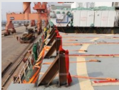
Stopper with pad at side edge to prevent pipe sliding.
