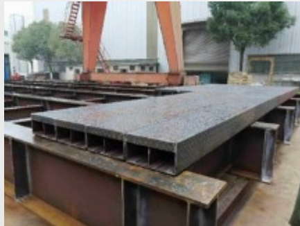
Trial Assembled Deck Panel.
