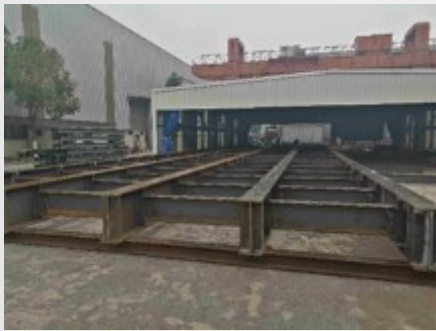
Trial Assembled Main Girders, Cross Beams and Splice Plate.
