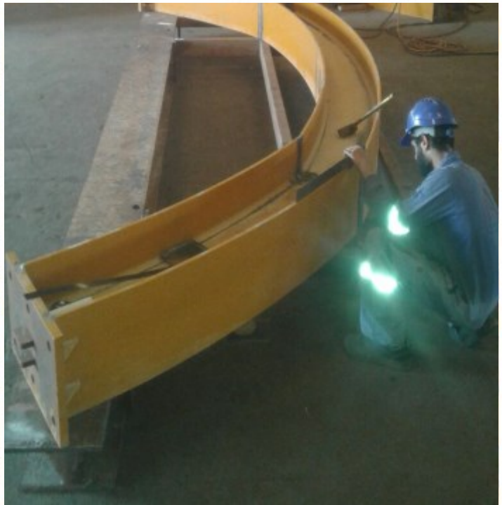
CIRCULAR WALING UNITS FABRICATION IN ESC YARD
